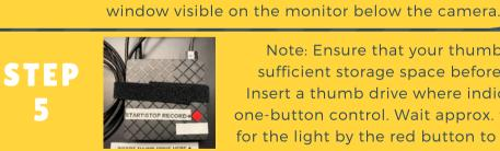
Note: Ensure that your thumb drive has sufficient storage space before recording. Insert a thumb drive where indicated on the one-button control. Wait approx. three seconds for the light by the red button to start pulsing.
